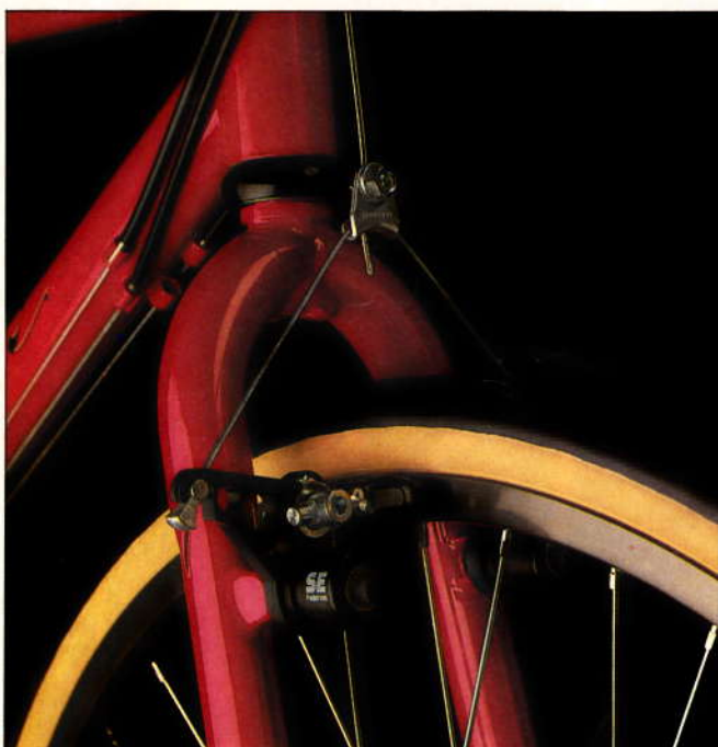
Ibis Type II fork allows precise control when the going gets gnarly; massive pivots on Scott Pedersen SE brakes contain self-energizers.
