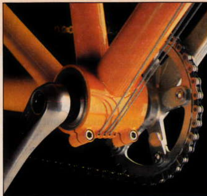
Front bottom bracket is stiffened by Jorgensen's Uptube design; unused cable guide is for optional rear disc brake.
