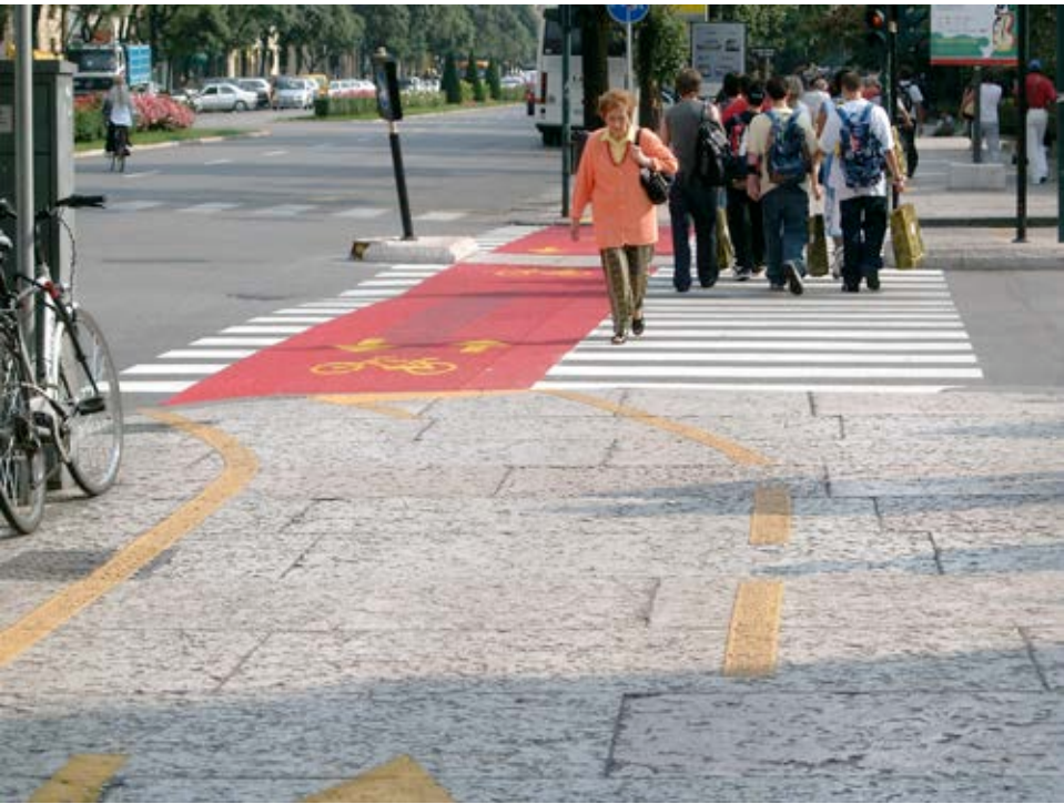
Munich Crosswalk A shared crosswalk with separate demarcations for bicycles and pedestrians will help keep crossing traffic sorted by mode at the BGT intersection with Brooklyn Avenue, University Way, and 15th Avenue.
