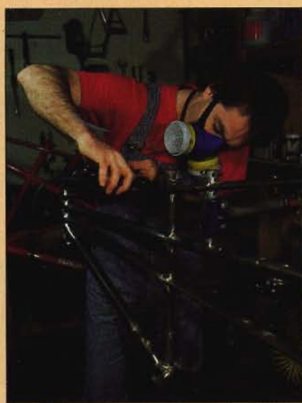
Jorgensen uses lugless brazing to join computer-selected tubing in all his framesets.
